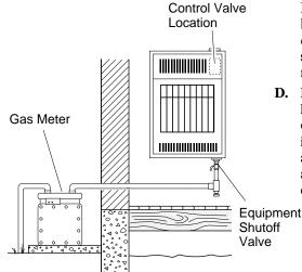
Figure 14 - Checking Gas Joints
